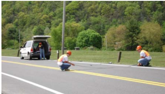
Figure 6. Graduate students place piezoelectric sensors in the lane.
